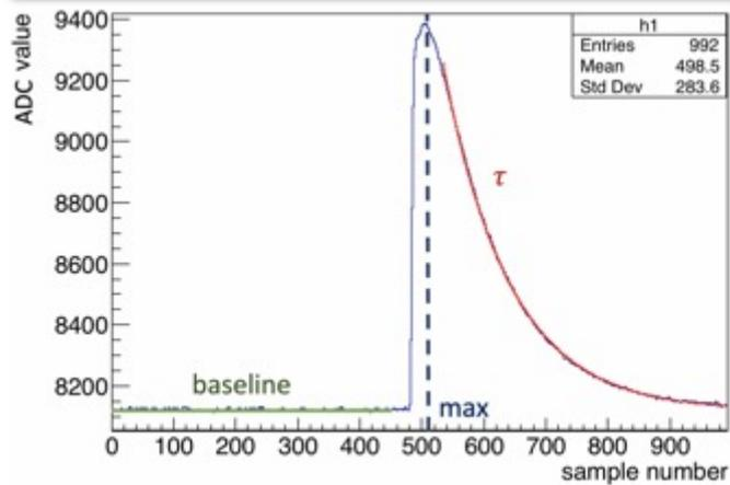
A trapezoidal filter (Jordanov filter) applied to the signal to extract the energy and time
